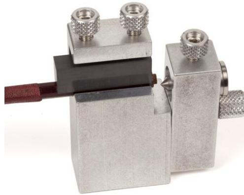
4. Bring the bushing guide into alignment with the bow while pushing the centering tool against the end of the bow, tighten the bushing guide thumb screw, and remove the centering tool.
