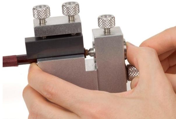
5. Insert a drill bushing with enough of a gap between it and the bow to allow for chips to escape and clamp it in place with the bushing thumb screw.
